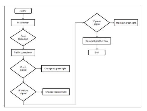
Figure 3. SATCS flow chart diagram.
