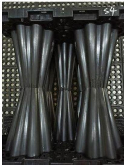
**Figure 3** Hollow cone shape column [5]
