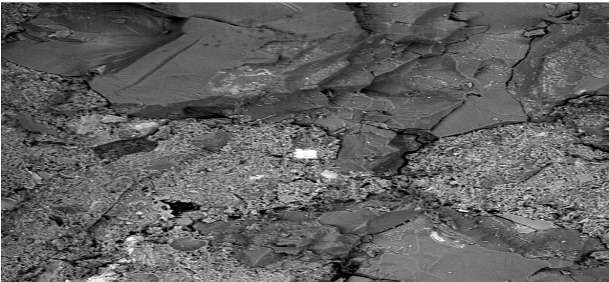
Figure 8 Micrograph of unmodified hot mix asphalt sample at 1000X magnification and 250µm magnification scale.
