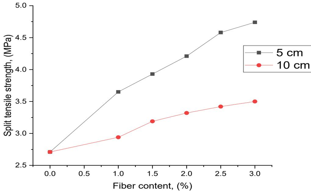
**Figure 10** Split tensile strength versus fiber content
