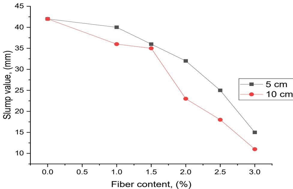
Figure 5 Slump versus fiber content of fresh concrete
