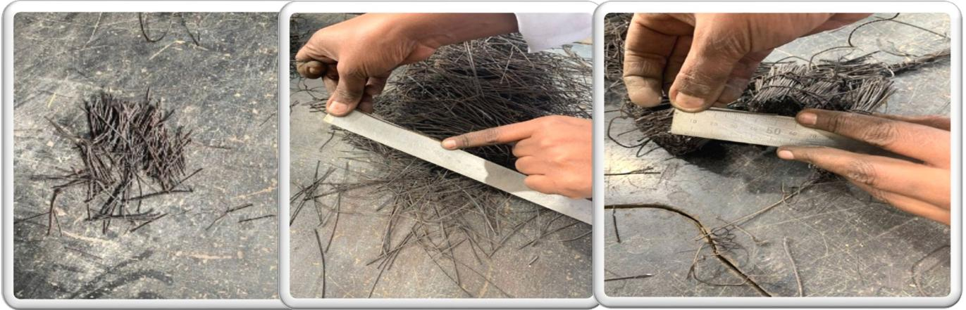
**Figure 1** Determining the length of fibers
