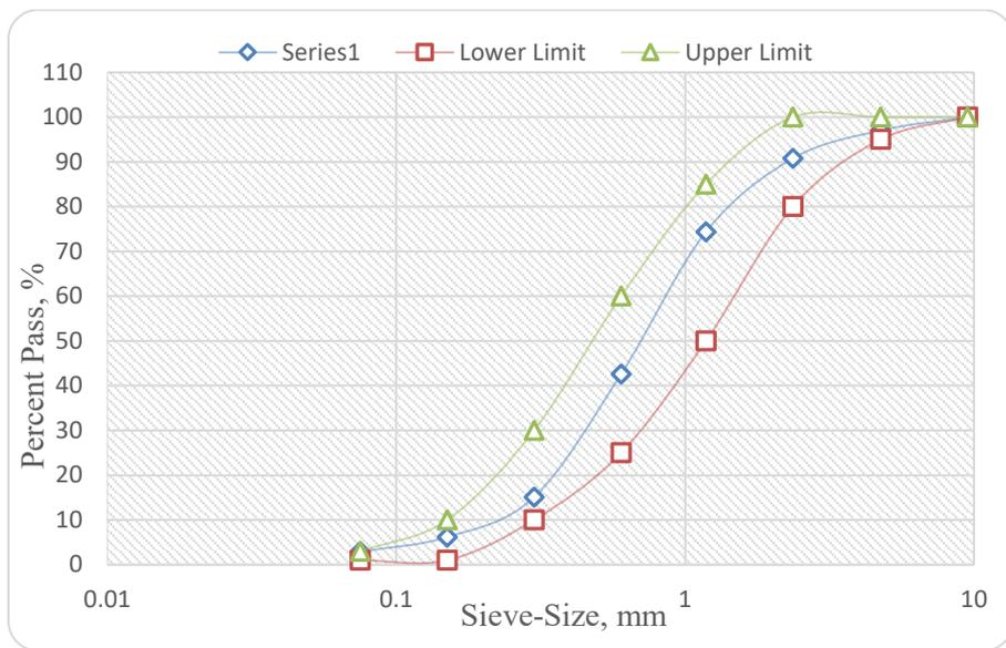
**Figure 3** Gradation of fine aggregate
