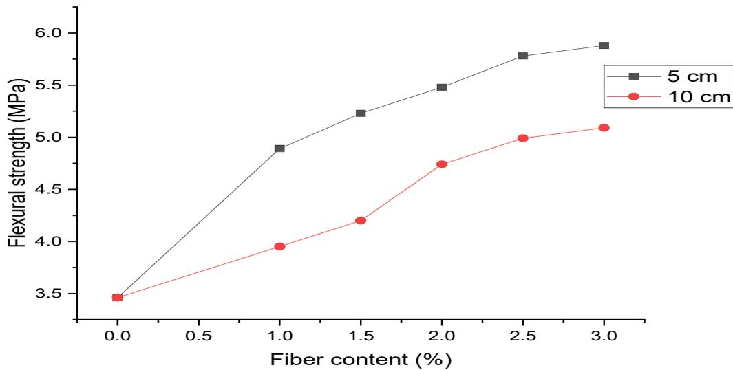
**Figure 9** Flexural strength versus fiber content
