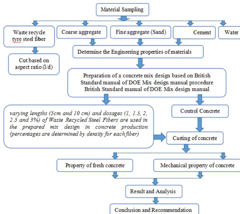
**Figure 4** Diagram showing details of the investigation pattern
