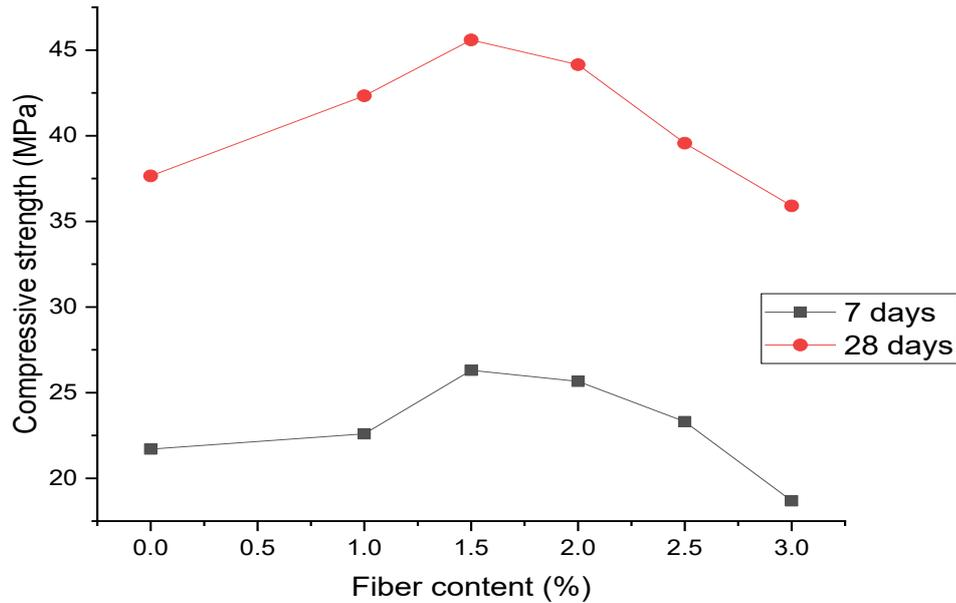
**Figure 6** Graph of compressive strength versus concrete with 5cm fibers
