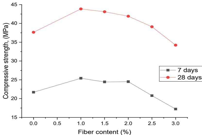
**Figure 7** Graph of compressive strength versus concrete with 10 cm fibers
