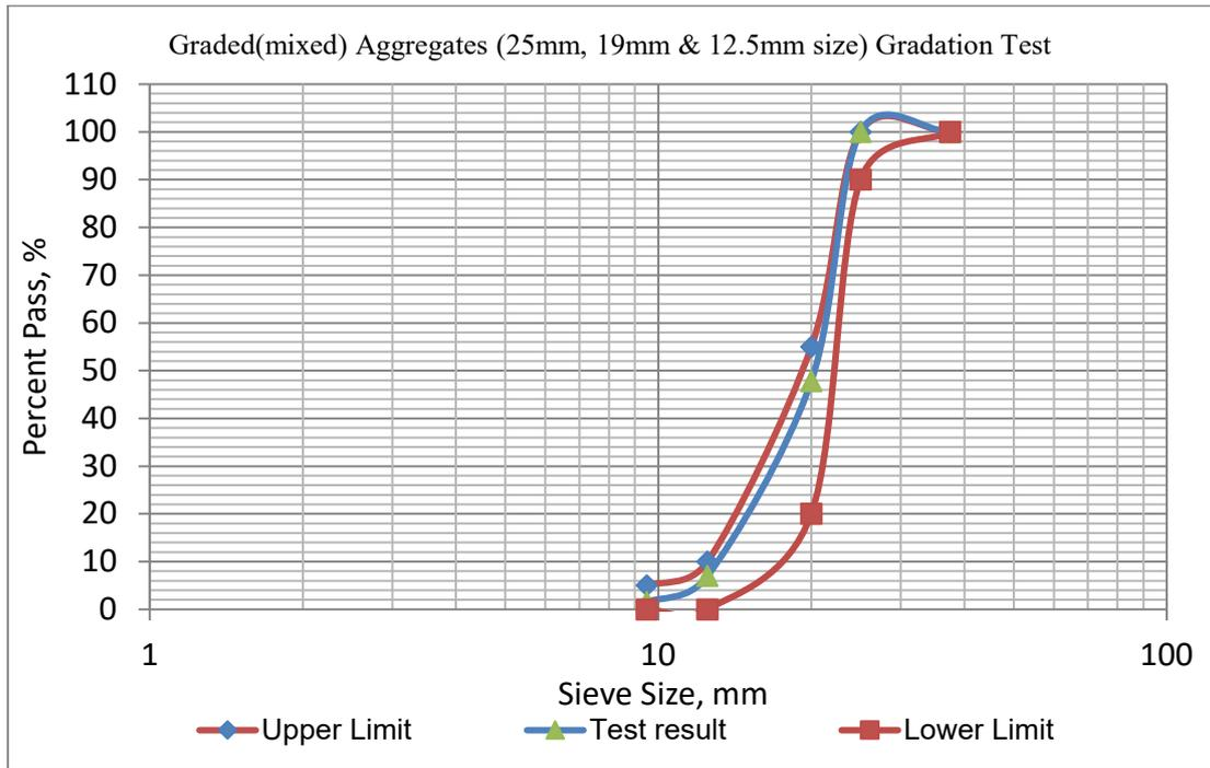
**Figure 2** Gradation of coarse aggregate
