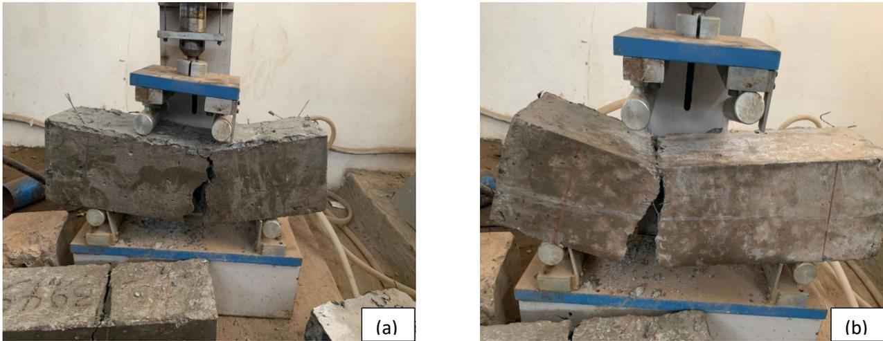
**Figure 8** Rupture of the concrete after testing a) for 5cm and b) for 10cm long RSFs
