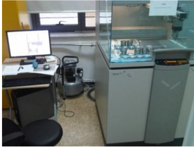
Figure 2 XRF spectrometer setup
