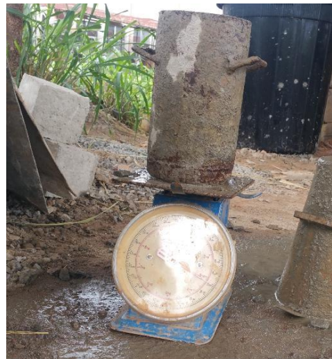
Figure 4 Compacting factor test
