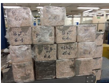
Figure 1 Sealed cubes in cling film for curing
