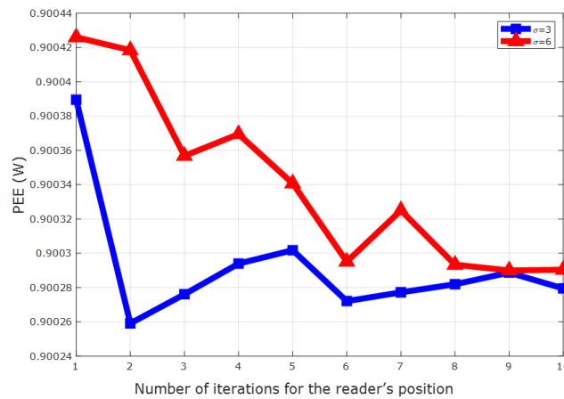
Figure 6: Absolute power estimation error as a function of the number of iterations for shadowing standard deviations \sigma=3\text{dB} and \sigma=6\text{dB} .
