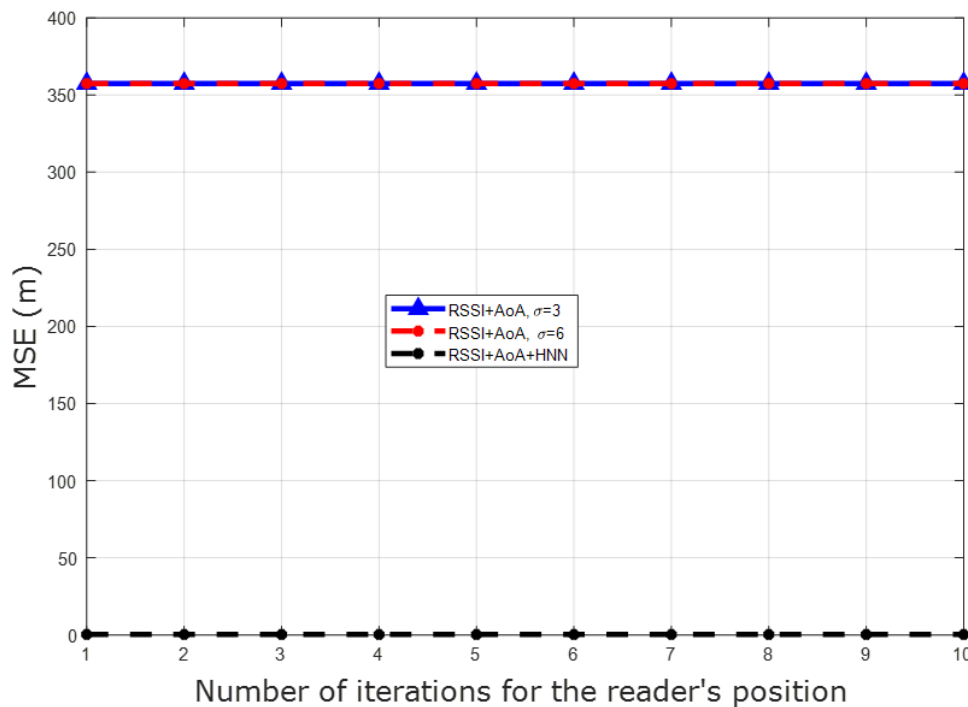
Figure 10: Comparison of overall performance between RSS/AoA and RSSI+ AoA+HNN based on the number of iterations for standard deviations \sigma=3\text{dB} and \sigma=6\text{dB}
