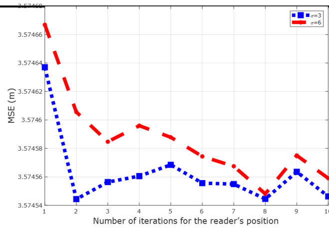
Figure 5: Mean square error as a function of the number of iterations for standard deviations \sigma=3\text{dB} and \sigma=6\text{dB}
