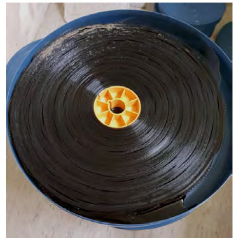
Figure 3: A film reel becoming host to common mould. This can potentially destroy the negative permanently rendering digitisation process useless
