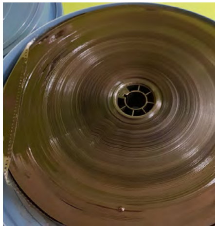
Figure 2: A film reel showing signs of vinegar syndrome . The film will stick to itself in the reel and becomes frail and easily flaked while emanating foul smell
