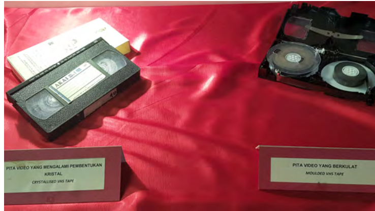
Figure 4. Two samples of old and possibly terminally damaged Video Home System (VHS) tapes afflicted with crystallisation and mould respectively
