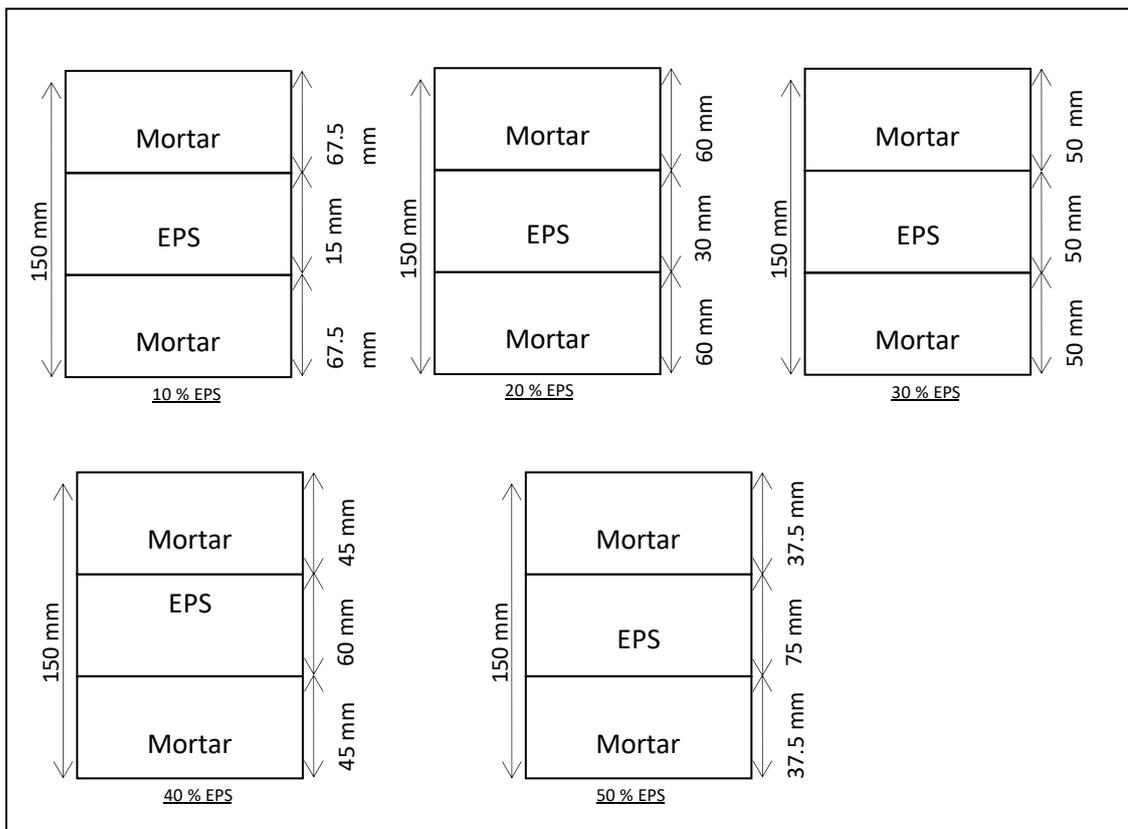
Figure 1. Layered mixing of EPS wastes
