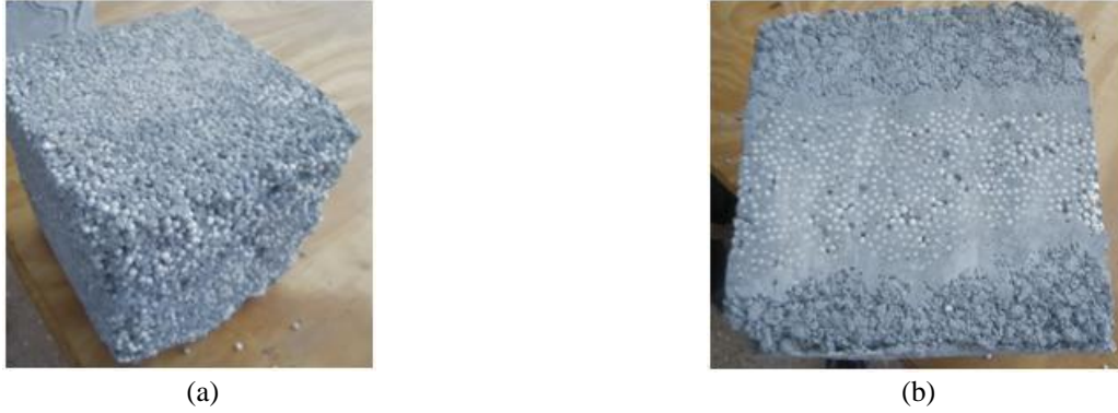
Figure 2: (a) Randomly mixed cube (b) and layered mixed cube
