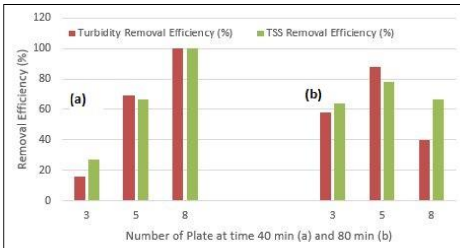
Figure 3. Effect of Number of Plate on Turbidity and TSS Removal Efficiency
