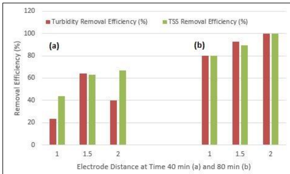
Figure 4. Effect of Electrode Distance on Turbidity and TSS Removal Efficiency
